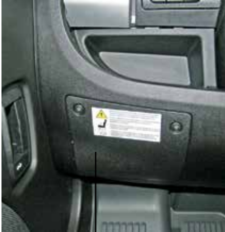
Original Fiat fuse box, under the dashboard on driver's side
