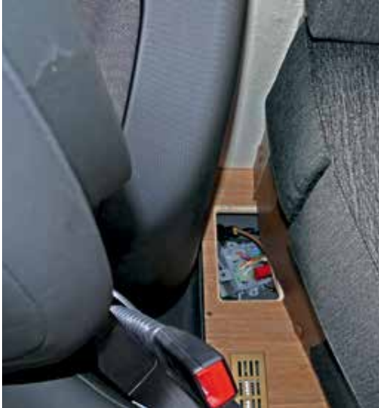
Additional fuse location of the vehicle electrics interface Fiat chassis electrics. Position intermediate floor area behind the passenger seat.
