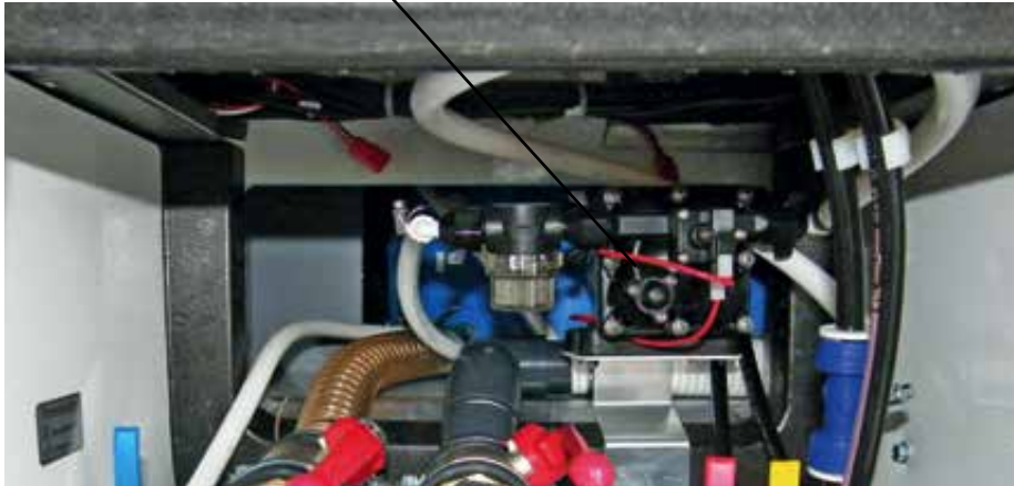
Position of water pump in supply space on driver's side
