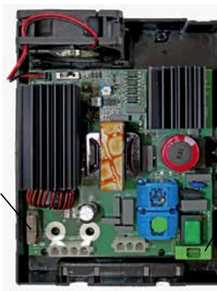
Protection electric currents output, 25A blade-type fuse
