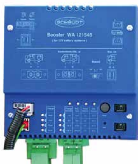
Booster WA 121545 (serial) charging set for leisure battery B2 while driving, charging capacity max. 45A
