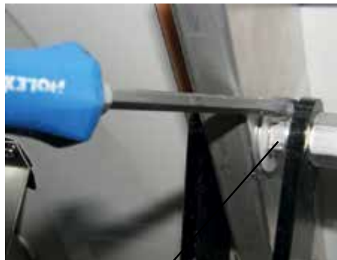
Round turned groove of the shaft (unlocked pos.)
