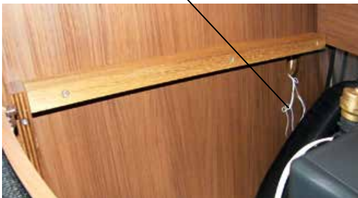
Emergency cord for mechanically unlocking the kitchen drawers
