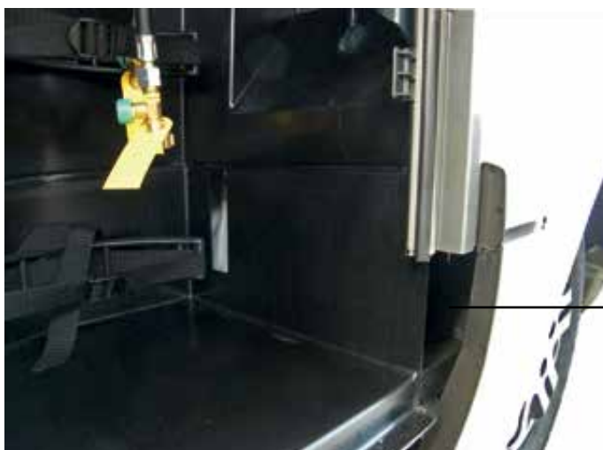
Gas bottle box on passenger side. Central position of gas supply
