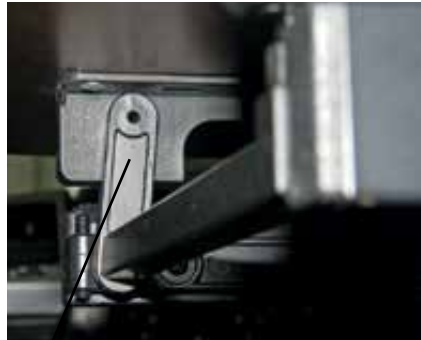
Vertical position = joint in push-in position
