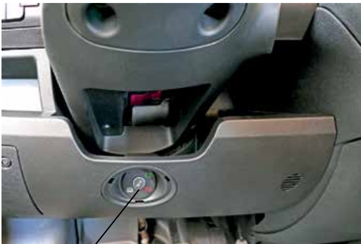
Vehicle battery section switch below the steering column
