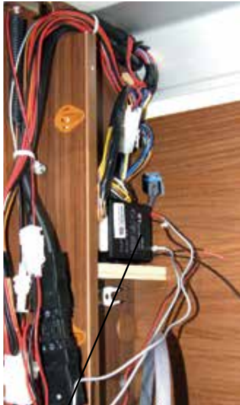
Position, alarm system control box in the side case, left wall cabinet
