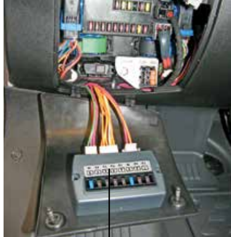
Fuse block, blade-type fuses of the additional switch panel
