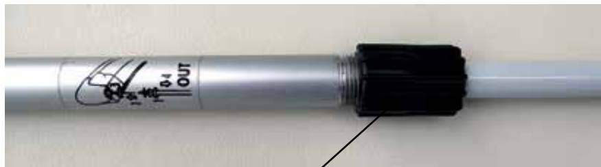
Loosened screw protection on the crank handle for telescopic linkage
