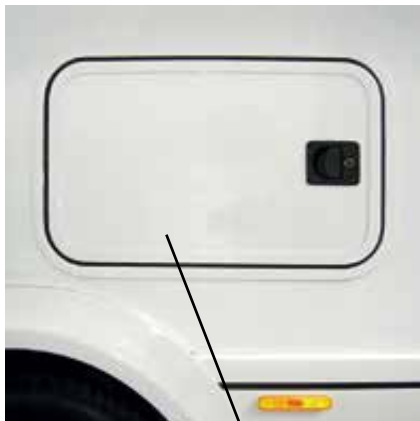
Fig. 2 Disposal door of the WC tank compartment, Model 2
