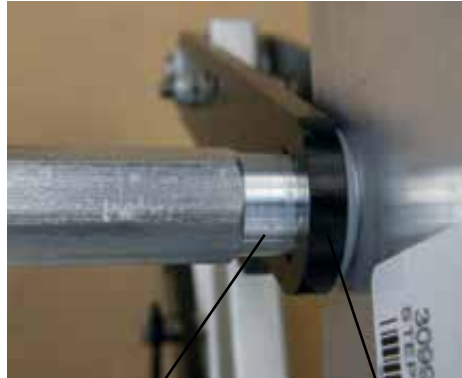
Round turned groove of the shaft (unlocked pos.)
