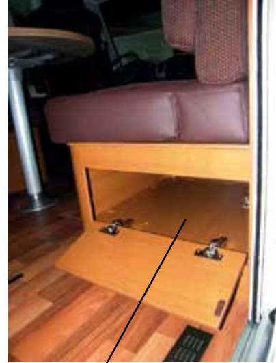
Bench storage space passenger side, model-dependent with lateral door (pressure catch lock)
