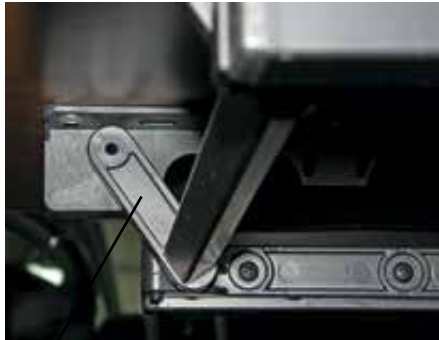
Inclined position = joint in extended position
