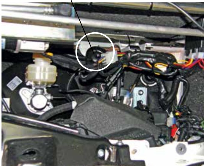
Alarm horn in engine compartment (position can vary)
