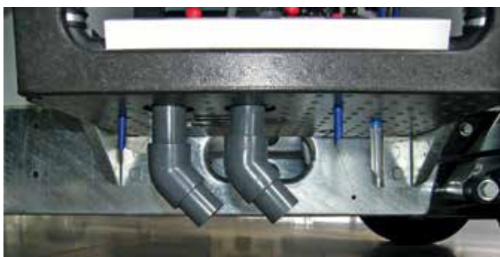
Discharge nozzle Water and waste water tank under the supply space
