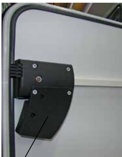
Servomotor on the lock case
