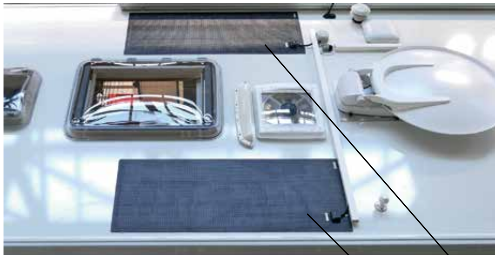
Glued to the roof surface, solar module mats
