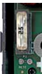
Protection electric currents output, 25A blade-type fuse
