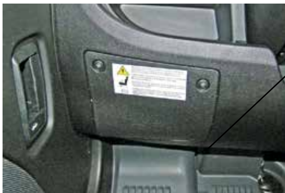
Position, remote control re- ceiver original Fiat ignition key, under the dashboard close to the Fiat fuse box
