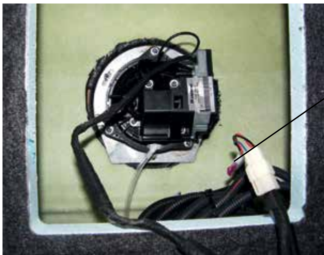
3A blade-type fuse at the cable loom, rear compartment
