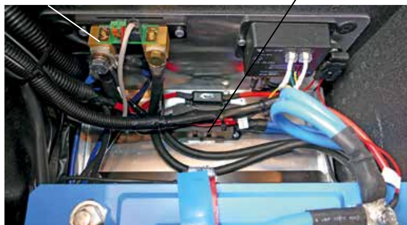
BMV Shunt 500A/ 50mV charger / inverter
