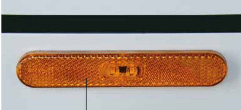
Side marker lamp glued
