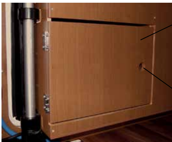
Disposal door with the cassette toilet swivelled out, access from the outside
