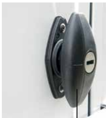
Handle lock in released position, in case of turnbuckle-lock mechanism
