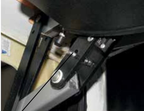
Linkage slack without nut, left side
