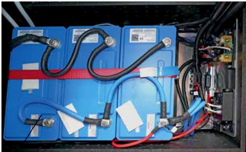
Lithium-iron-phosphate-batteries, mounting location lower level of the floor at entrance height
