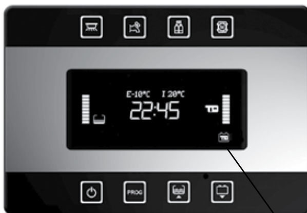
Alarm symbol, first leisure battery discharge stage
