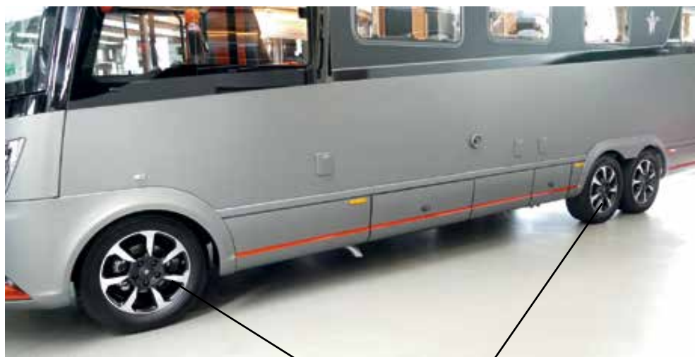
GSM12 16" light alloy wheel rims on front and rear axle
