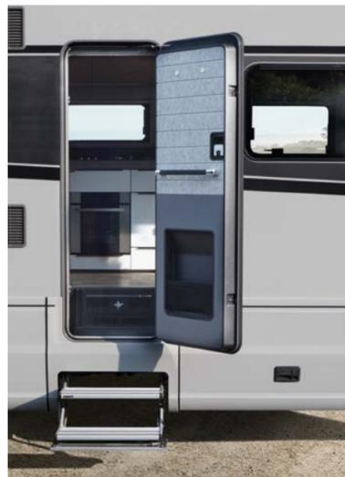
For trouble-free loading and unloading of the drawer units, we have equipped our body door with smart sensor technology. When the storage flap is open, the body door opens no further than 90°. This keeps the door and flap from colliding and is what makes such a large storage space next to the door even possible. It's unique technology that we have registered for a patent.
